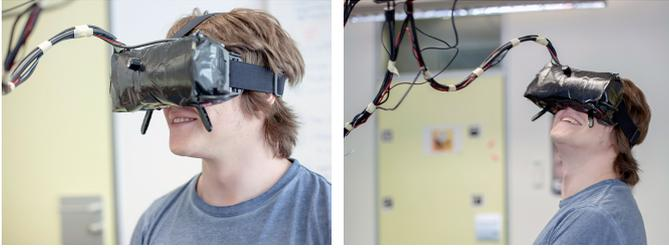
Fig. 2. Our experimental setup: A participant is watching an immersive video using our custom-built head-mounted display with integrated eye tracking. The participant is seated on a rotatable chair, in order to allow safe and free 360° body and head movement.
